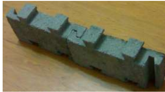
Fig. 2. The multi-functional adobe
